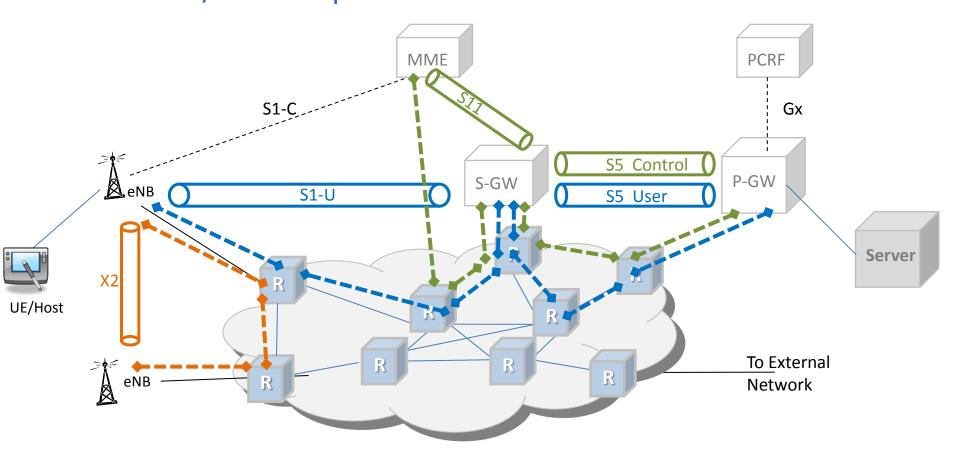
More than 1 tunnel between policy enforcement points. Example: UE PDN connection traverses [eNB] << S1-U >> [SGW] << S5/S8 >> [PGW].
